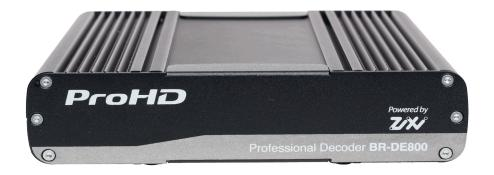
The ProHD BR-DE800 Streaming Decoder is a high-performance IP decoding appliance for standard definition and high definition MPEG-2 and MPEG-4 H.264 streams, ideal for use with JVC streaming cameras including the GY-HM200, GY-LS300, GY-HM650, GY-HM850 and GY-HM890 cameras. The decoder features a flexible selection of output interfaces, including 3G, HD-SDI, HDMI and Composite video.
