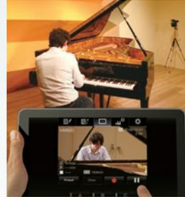
The camera on the stage can be remote controlled from a smart device. Controls include REC/STOP, Zoom, Focus, Iris and more detailed settings while viewing live images from the smart device screen.
