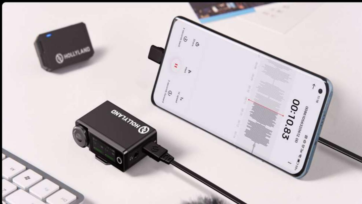
Simply connect the receiver to a mobile phone with the included MFi-certified USB-C to Lightning cable or USB-C to USB-C cable or the optional 3.5mm TRS to 3.5mm TRRS cable. Achieve real-time audio playback on your phone speaker without the need to unplug the receiver from your device for an immediate audio quality check.
