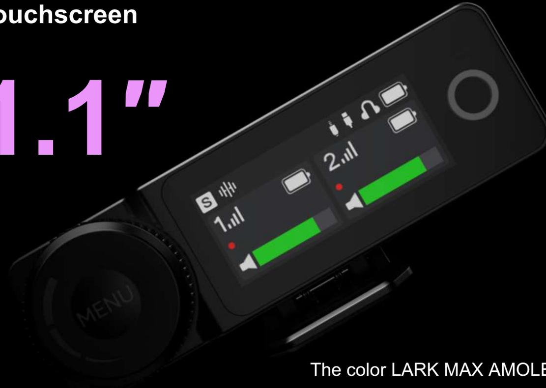
The color LARK MAX AMOLED touchscreen allows you to adjust transmitter settings and provide a real-time visual check of the power supply, signal, audio level, connection status, and more.
