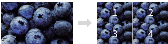
4K 2 Sample Interleave (2SI) : Pixel based segmentation
