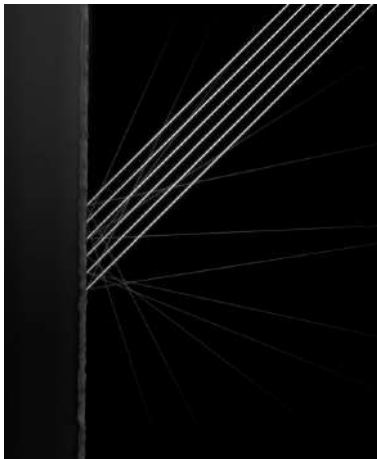
Light scattering on nano-texture cover glass
