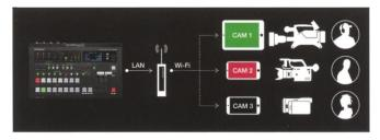
Roland's unique and proprietary wireless tally system uses a wireless LAN router connected to the V-60HD to send tally information to iOS or Android devices on the network.
