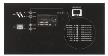
Assign up to eight analog audio inputs a separate audio embed channel on SDI 1 and 2 outputs, for a separate mix pre-effect (dry) or post-effect (wet) for correcting audio problems post live event.
